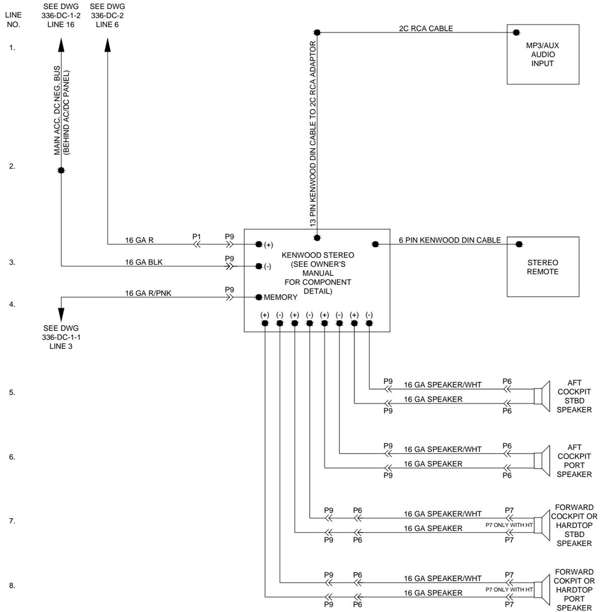
*12 Volt DC with Satellite Radio Diagram*
